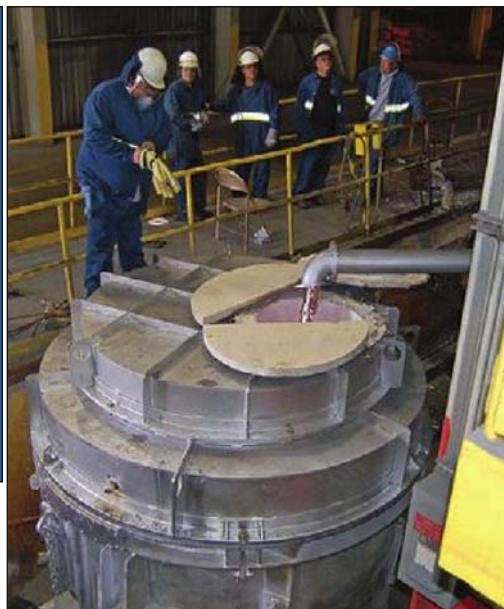
Figs. 1 and 2. Apogee's transportable electric ladle features baffle or side pocket panels with embedded high-intensity electric resistance elements.
