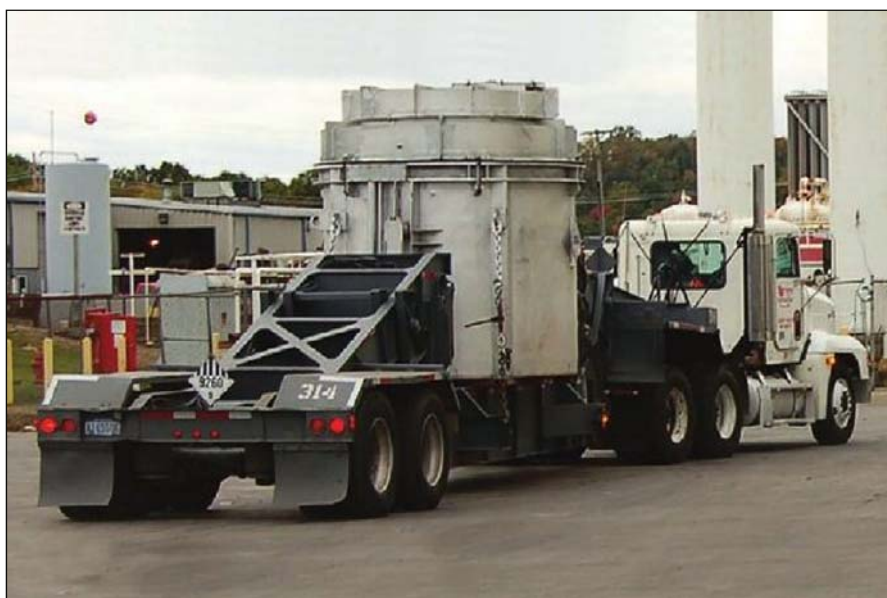
Fig. 3. The ladles come in a range of sizes and designs, including this 22,000-lb.-capacity ladle for road transport.
