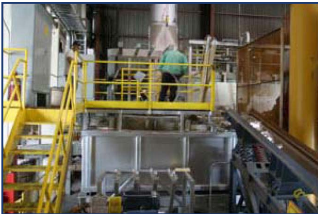
A 7,000lb commercial prototype ITM was commissioned for Aleris Rolled Products at their Newport, OH facility. This unit is capable of a 5,000lb/hr output when melting light weight scrap (edge trim), and up to 7,000lb/hr solid charge.
